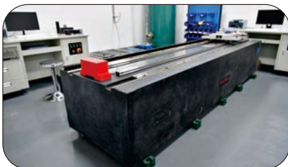
Linear guide complex performance Test Equipment
