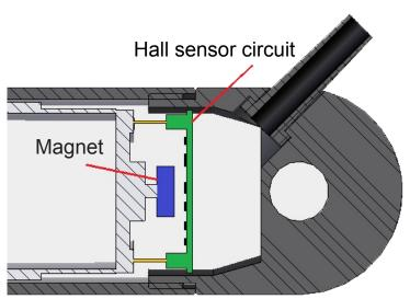
The hall sensor option is available for all three Bansbach actuator models. The hall sensor enables control of the position of the piston rod very precisely. Furthermore, the hall option allows driving of two or more actuators synchronously, depending on the choice of controller. A combination of the above features is of course, also possible. The PCBA is fully backwards compatible with earlier versions. Previous versions have a limited supply voltage range.
