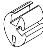
Gasket US-838 Other dimension available on request Material EPDM
