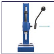
Manual lever can be refitted for right and left-handers
