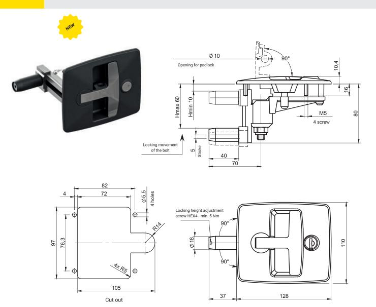
Sealing of lockable doors by folding the lock handle into the lock body. The locking height (dimension H) is adjustable from 10 to 60 mm. Locking height is adjusted when the lock is installed and locked with the HEX 4 key - Recommended tightening torque for the adjusting screw: 5 Nm.
