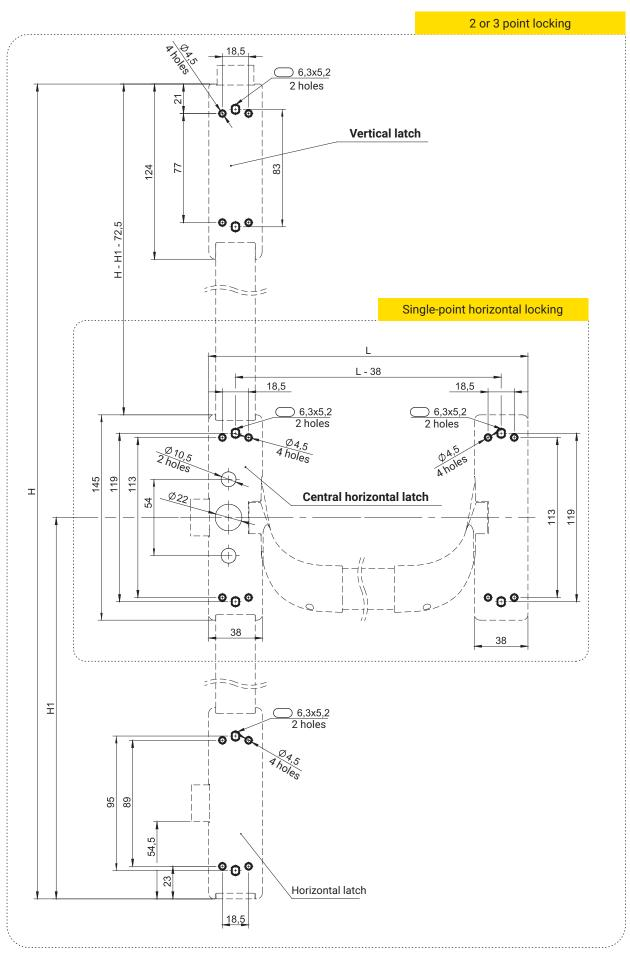
Each lock can be mounted on 4 holes Ø 4,5 or 2 holes 6,3x5,2
